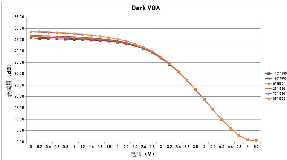
MEMS VOA temperature attenuation curve: the horizontal coordinate is voltage (V), and the vertical index is VOA attenuation value (dB).
