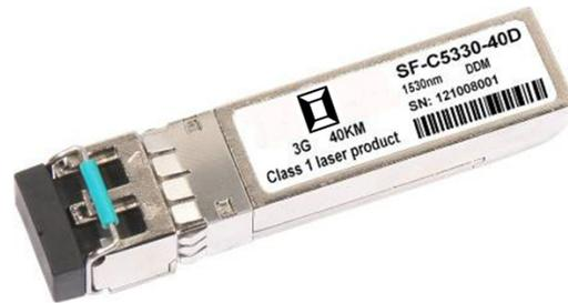
The optical output can be disabled by a TTL logic high-level input of Tx Disable, and the system also can disable the module via I2C. Tx Fault is provided to indicate that degradation of the laser. Loss of signal (LOS) output is provided to indicate the loss of an input optical signal of receiver or the link status with partner. The system can also get the LOS (or Link)/Disable/Fault information via I2C register access.
