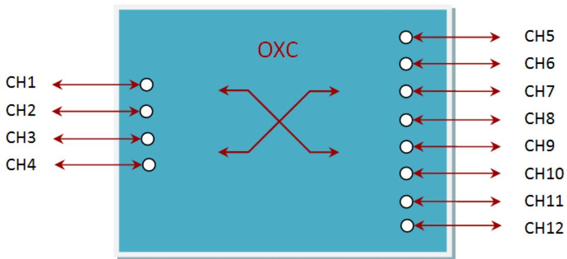
There are 12 ports of CH1~CH12, and any two ports can be intercommunicated. For example,
