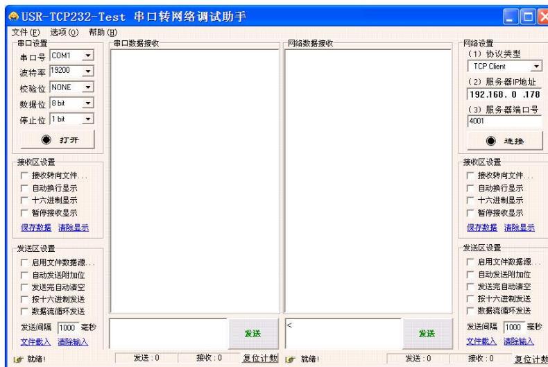
USR-TCP232-Test interface of serial port to network debugging assistant
